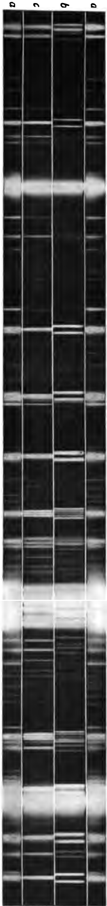
EFFECT OF MAGNETIC FIELD UPON THE SPARK SPECTRUM OF TITANIUM. Experimental conditions varied to bring out both strong and weak lines. a. Spark without field. b. n -Components. c. p -Components.
